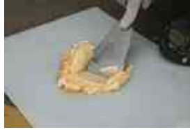
3. The epoxy is squeezed from the cartridge and mixed.
